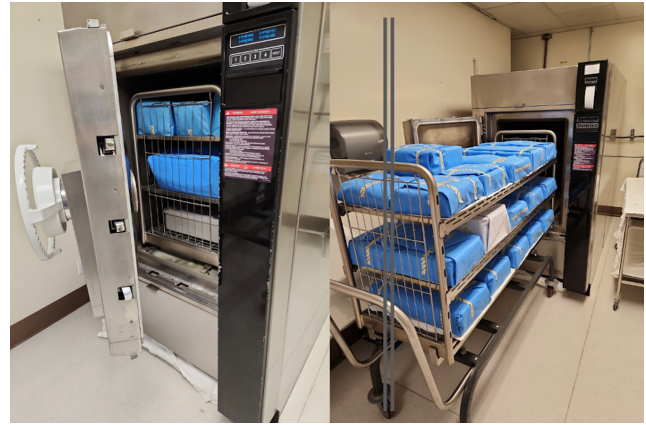
Figure 9. Initial cooling starts with the autoclave door left ajar and contents left inside for 15-45 minutes. This starts the gradual room temperature cooling process. Subsequently, the contents are pulled in front of the autoclave without touching for additional progressive cooling. Total cooling can take 0.5-2 hours of more. Inappropriate rapid cooling can cause condensation and compromise sterility. Autoclaves are indisposed during the initial cooling phase due to the limitations of the porous barrier creating autoclave use inefficiencies.
