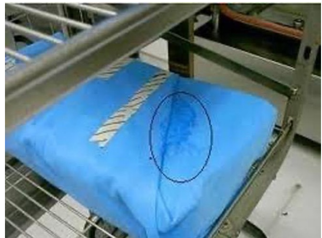
Figure 10. Rapid cooling can cause droplet condensation, dripping and focal wet spots which can wick in bacteria and compromise sterility of the porous barrier and its contents.
