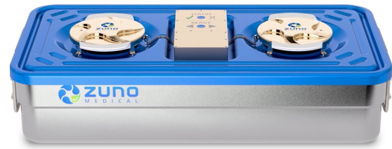
Figure 15. A smart sterilization container forgoes the porous barrier by capturing a vacuum seal within the autoclave with electromagnetic technology. The digital container possesses electronics that sense temperature, pressure and moisture. After appropriate exposure and during the subatmospheric terminal drying phase within the autoclave, magnetic valves are activated capturing a sterile vacuum seal. No porous barrier is necessary.
