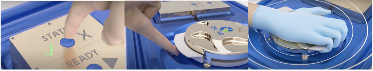
Figure 16. A digital smart container creates a verifiable vacuum seal that can be checked at any point before surgery. First, a press of the button electronically visually confirms an intact vacuum seal with a green checkmark. Second, finger palpation confirms a physically intact seal. These two checks can be performed at any time before surgery. Third, at the time of surgery, the vacuum seal is broken and confirmed audibly.
