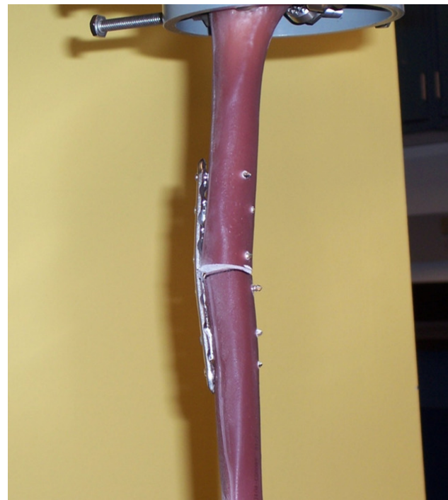
Figure 4. 4.5 mm plated humerus following failure testing.
