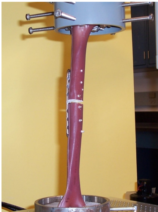
Figure 3. 3.5 mm plated humerus following failure testing.
