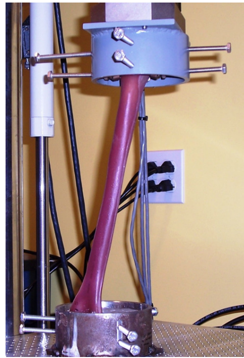
Figure 1. Humerus Prepared for Stiffness Testing.
