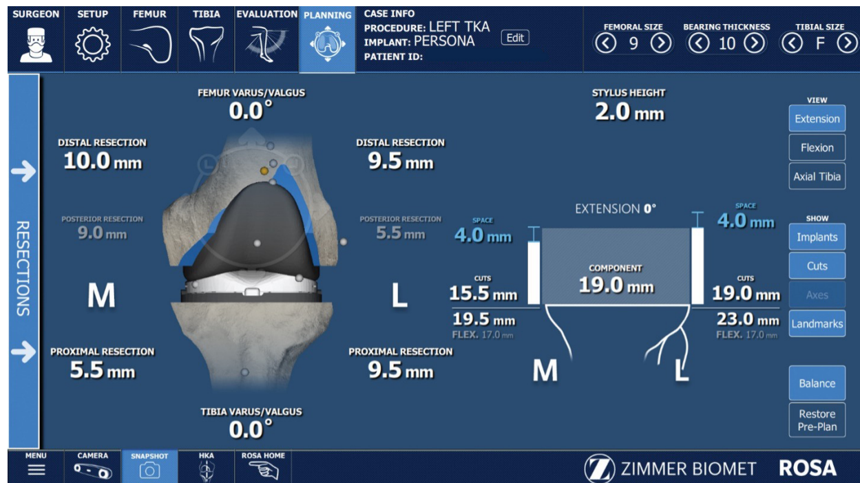
Figure 3a: Illustration of ROSA TKA planning and gap balancing tool used pre- and intra-operatively to allow for the limb alignment, gap balancing, and femoral rotation to be adjusted using objective, real-time data.
