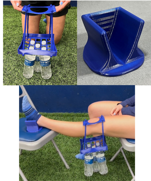
Figure 3. Top Left: Assembled knee extension device with water bottles attached as weight. Top Right: Foot holder. Bottom: Knee extension device in use with weight suspended under the knee.
