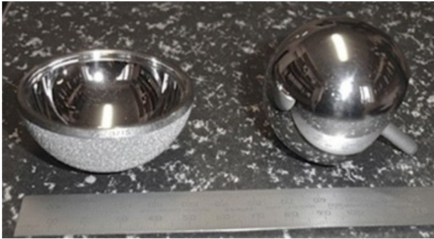
Figure 2. DePuy ASR metal on metal resurfacing hip (Wienroth, McCormack, and Joyce 2014).
