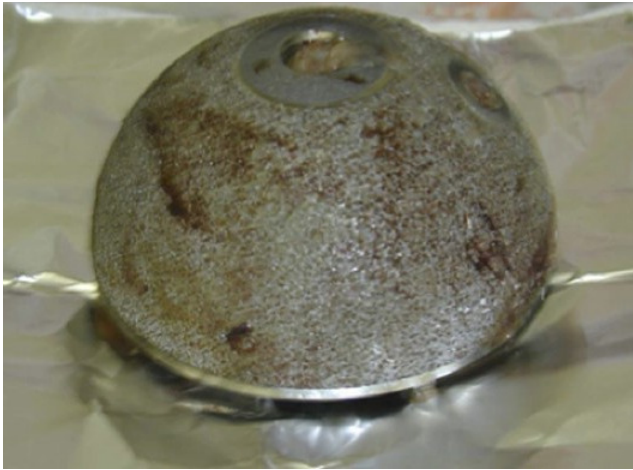
Figure 1. An explanted Inter-Op cup after 11 weeks in vivo showing no bone ingrowth and a red and gray gel-like residue (Wyss 2019).
